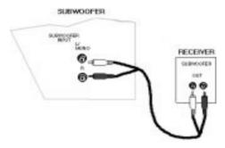
NOTE: A receiver with a single output should be connected to the input labeled L/MONO.
